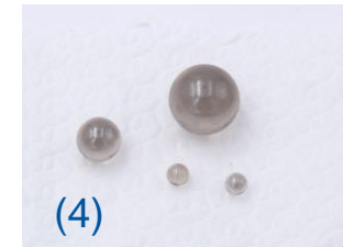
High index glass balls for high precision alignment optical systems: (1) not irradiated, (2) 300 kGy, (3) 1 MGy and (4) 5 MGy Gamma irradiation in BGS facility conveyor, September / October 2018
