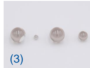
High index glass balls for high precision alignment optical systems: (1) not irradiated, (2) 300 kGy, (3) 1 MGy and (4) 5 MGy Gamma irradiation in BGS facility conveyor, September / October 2018
