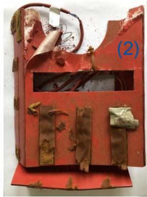
Vacuum bake out jacket: (1) not irradiated, (2) 10 MGy Gamma irradiation in BGS facility conveyor, May / June 2017
