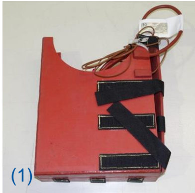
Vacuum bake out jacket: (1) not irradiated, (2) 10 MGy Gamma irradiation in BGS facility conveyor, May / June 2017
