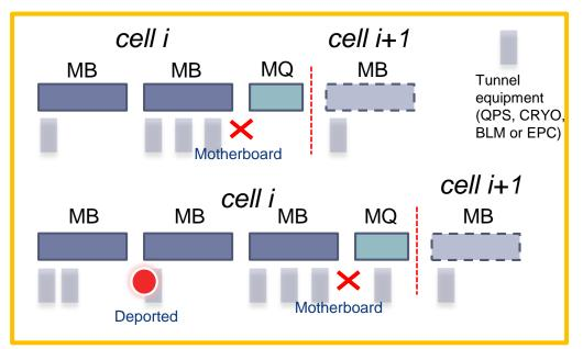
**DS/ARC (from cell 7 to 20)** RadMon are placed **below the interconnect** between the last MB/MQ of a given cell
