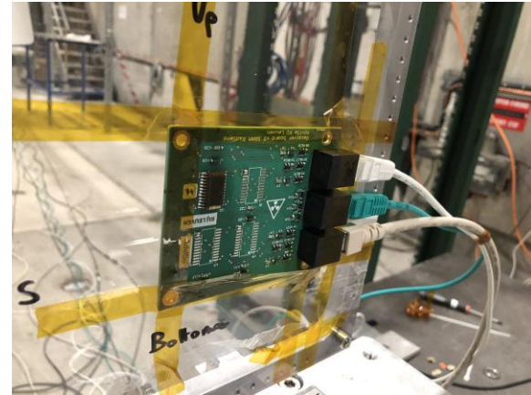
SRAM-based SEU Monitor at H8 (Credit: Jialei Wang)
