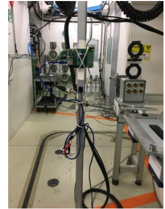
CHARM Radiation tests of SF2 ©Courtesy of G. Gnemmi
