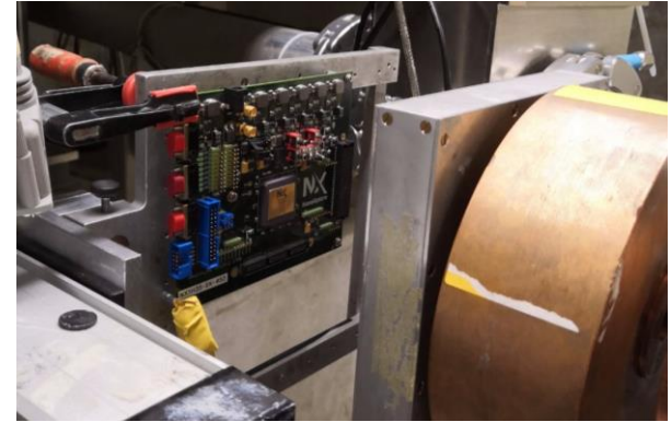
NG-MEDIUM FPGA Radiation testing at PSI facility with 200MeV beam
