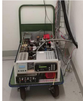
Test bench with MKS baratron reference
