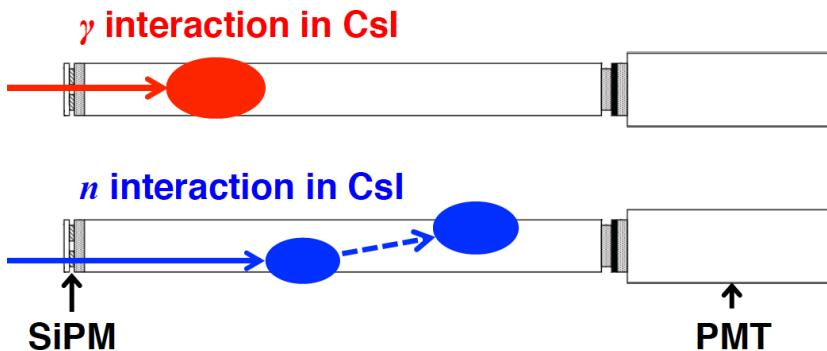
Resolve  $\gamma/n$  interaction depth by reading light from front CsI face with SiPM
