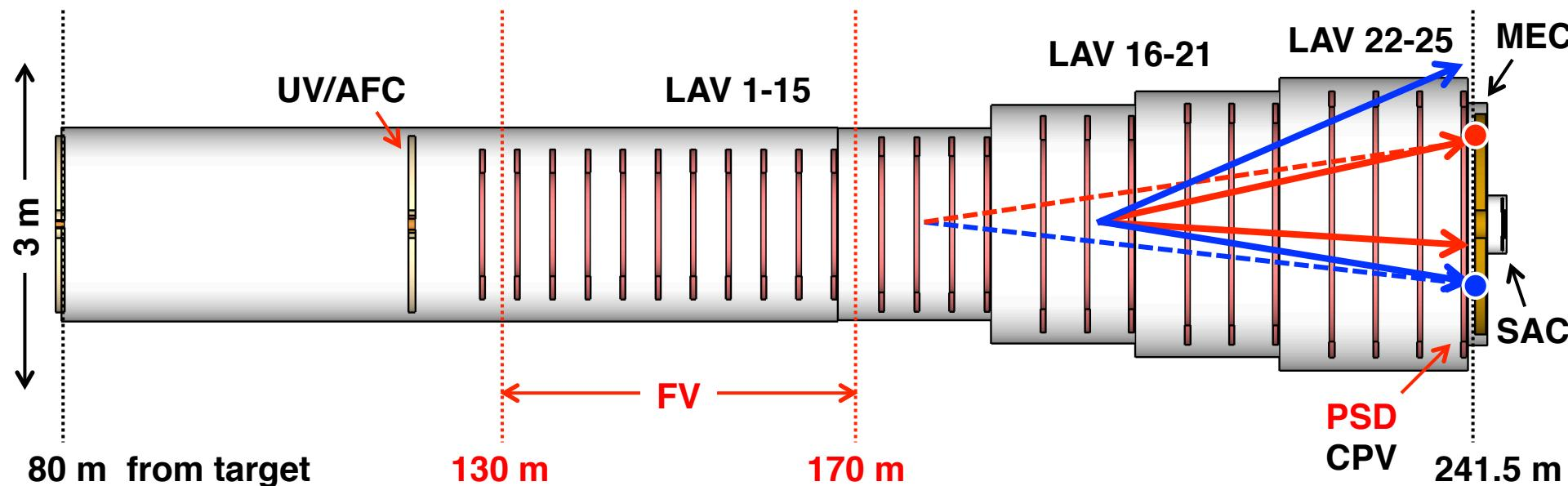
**Distance from FV to LKr significantly helps for rejection of “odd” background**
