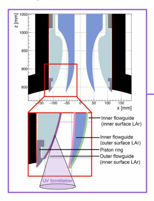
Po210 α-decays from the surface of acrylic flowguides located in the neck contribute to the background rate at low PE. Requires LAr located in close proximity to flowguide surfaces (e.g. a thin LAr film).
