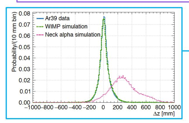
Left: Difference between the reconstructed z-position returned by the time residual-based fitter and the PE fitter (shown: z(time) – z(PE)).
