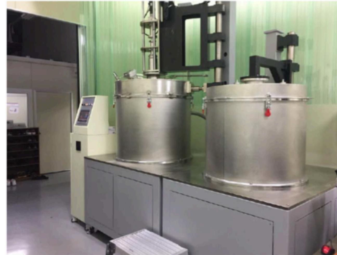
~ 100 kg NaI crystal (ingot) grower
