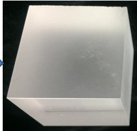
LYSO cube grinded on 5 sides and polished on 1 side
