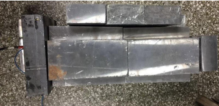
Lead shielding room(thickness ~10cm)
