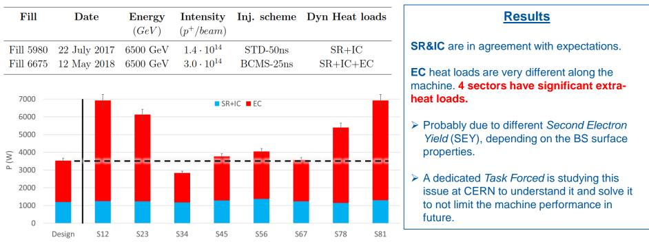
BS dynamic heat loads at 4.6 K – 20 K on the 8 LHC sectors for Fill 6675 compared to LHC Design report
