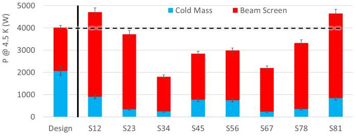
Total equivalent dynamic heat loads at 4.5 K on the 8 LHC sectors for Fill 6675 compared to LHC Design report
