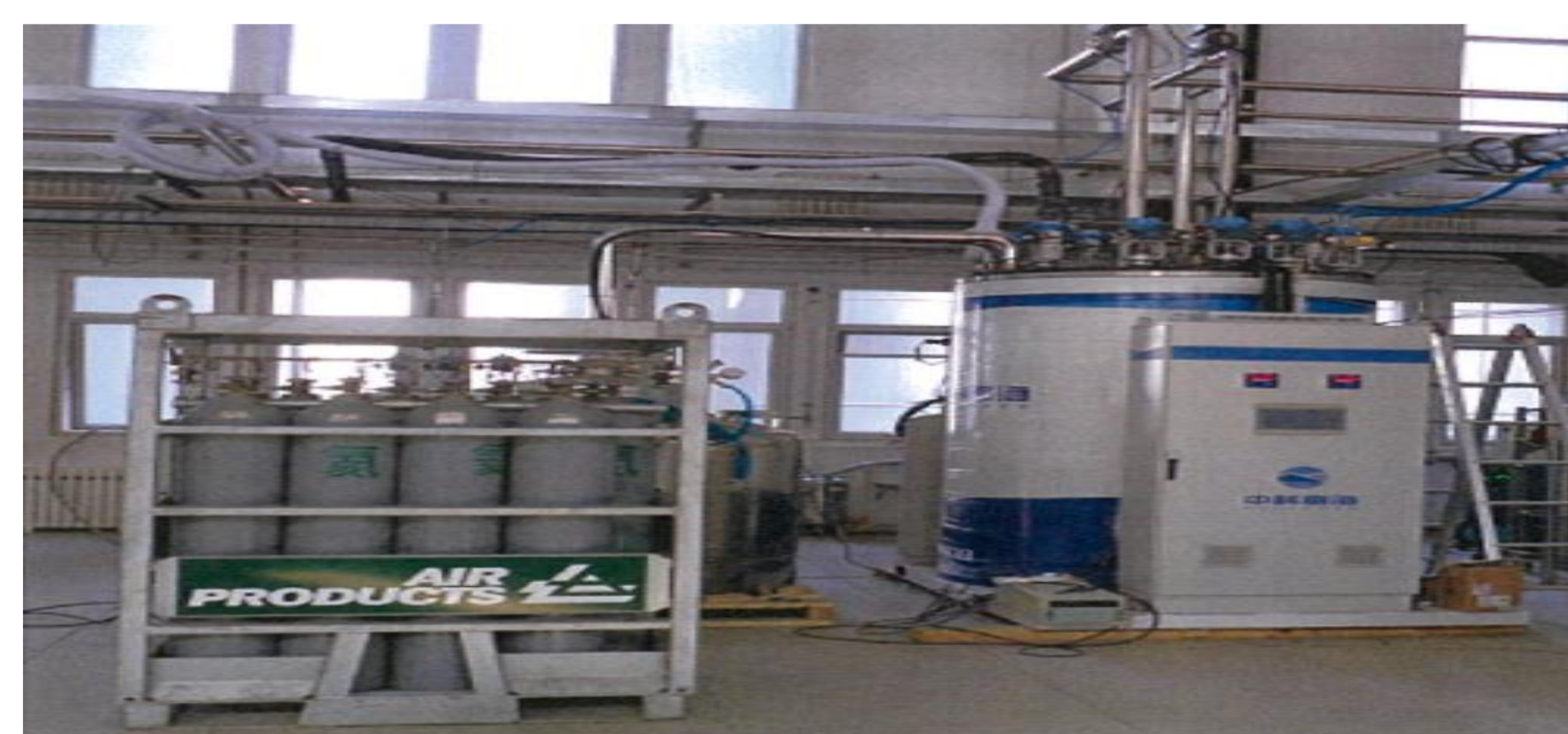
Figure 2. Physical diagram of the cold box and the Dewar
