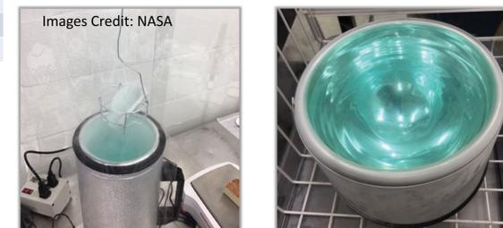
Aerogel specimen under LO<sub>2</sub> boil-off calorimetry testing used to calculate TCH
