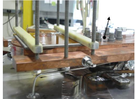
Figure 4. Sample test arrangement with samples clamped directly to cold plate and sample bottom with foil heaters.
