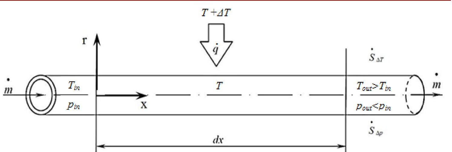
Heat transfer generated entropy can be calculated from Eq. 2. The entropy stream is increasing with the decrease of the process pipe temperature what makes this entropy source especially important in cryogenic conditions. Because this work uses entropy analysis to compare two support systems for process pipes in cryogen transfer lines having equal length, equal process pipe diameters and equal cryogen flow rates, the entropy fluxes generated due to flow resistances are equal in both cases.
