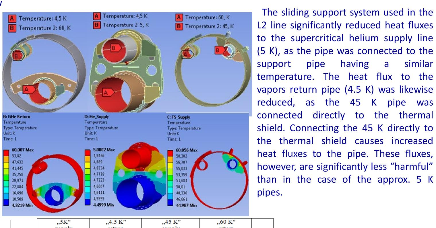
L2 line significantly reduced heat fluxes to the supercritical helium supply line (5 K), as the pipe was connected to the temperature. The heat flux to the vapors return pipe (4.5 K) was likewise connected directly to the thermal shield. Connecting the 45 K directly to the thermal shield causes increased heat fluxes to the pipe. These fluxes, however, are significantly less "harmful" than in the case of the approx. 5 K
