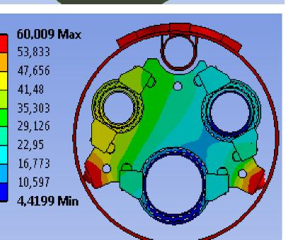
The sliding support used in this model pipes a temperature of approximately 5 K with pipes for thermal shield cooling, which have temperatures of 45 K and 60 K. Such a connection results in heat flux in the location of the support, from the 45 K and 60 K pipes to the approx. 5 K pipes, causing negative entropy fluxes in the pipes for thermal shield cooling.
