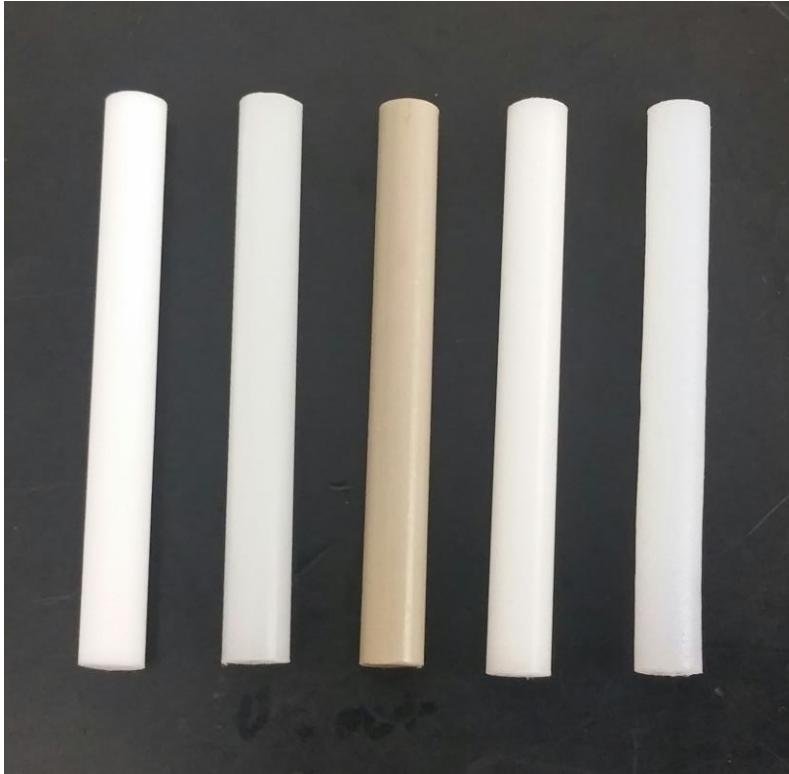
Typical 6cm posts that were soaked in Xenon and Argon
