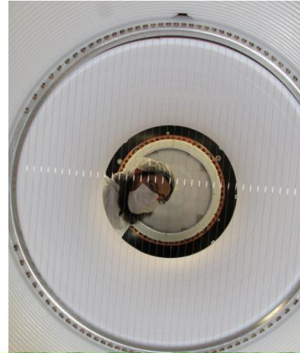
HDPE field cage + teflon reflector
