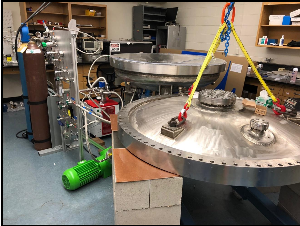
High Capacity vessel for testing large scale EL regions
