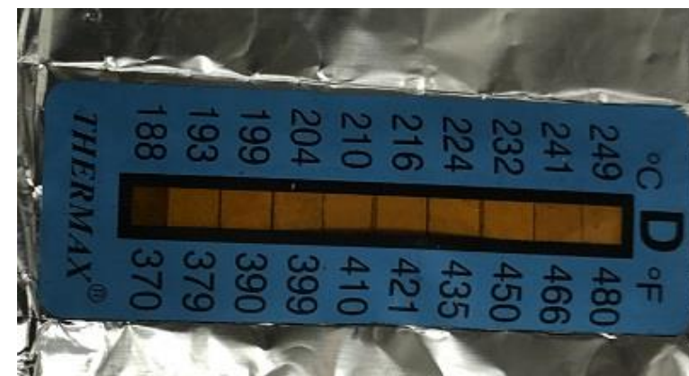
The temperature in the chamber after 300min copper deposition is 188 centigrade.
