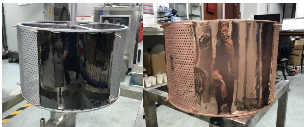
Before copper deposition (left). After copper deposition (right).
