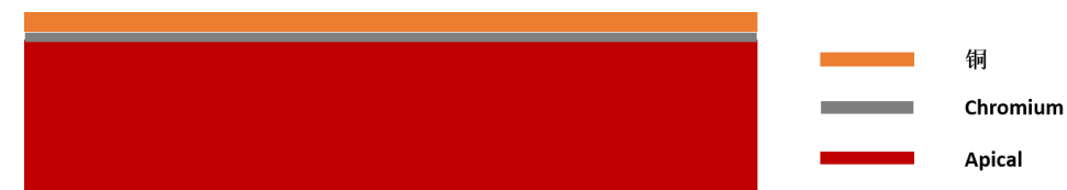
Structure of APICAL substrate
