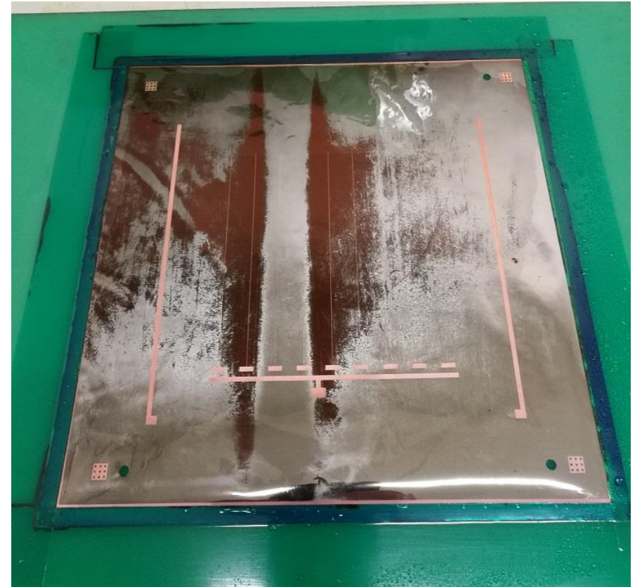
Etching chromium of the \mu RWELL PCB
