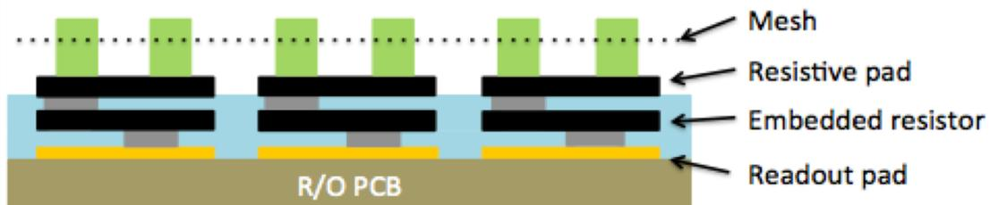
Resistive pad to anode pad Resistance: ~3-7 MOhm
