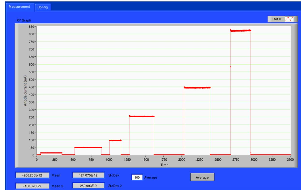
Confirmation of negligible (or unmeasurable) charging-up up to  $10 \text{ MHz/cm}^2$  (in this plot rates up to  $\sim 1 \text{ MHz/cm}^2$ )
