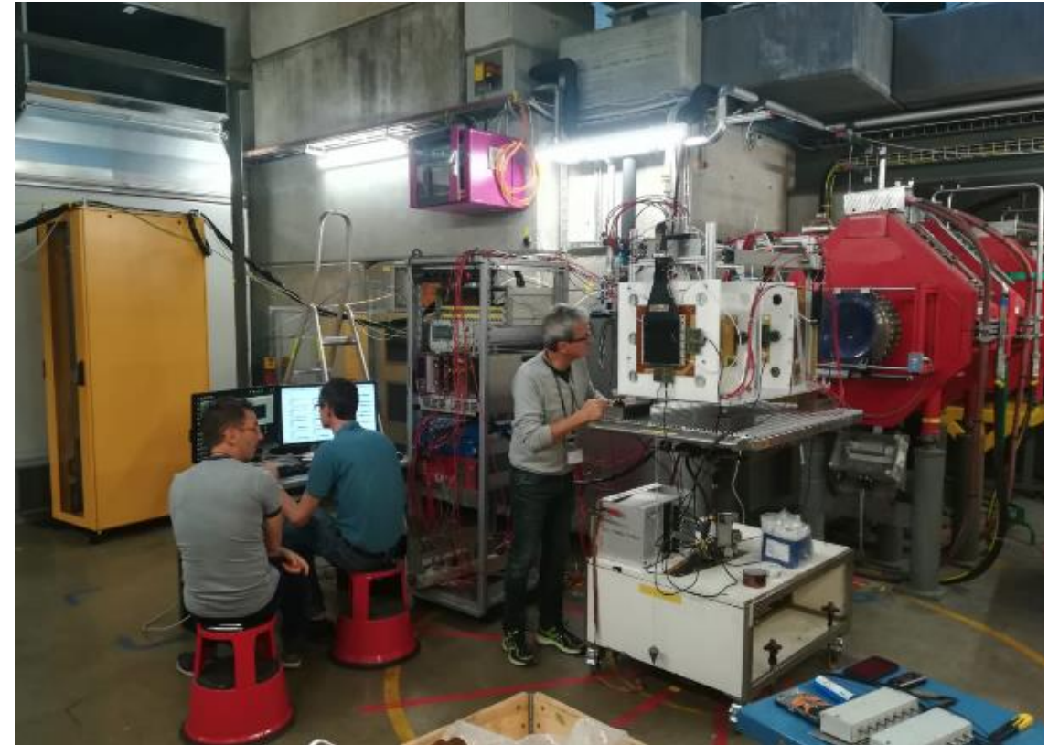
Our setup in \pi M1 area: a tracker system + 10 \mu -RWELL on a movable XYZ table + rack+SRS+ power supply, etc
