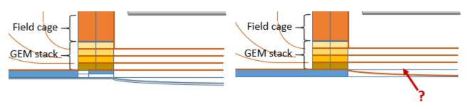
Readout in four quarters read from all four sides VMM3a hybrids perpendicular to readout plane → needs to be folded around detector edge New 140 Pin Hirose connectors
