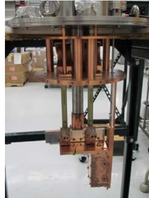
Design model (top) and a photo (bottom) of experimental setup based on a cryocooler, to measure AC heating in SCAPE magnet.
