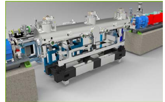
Design model of APS-U straight section with an SCU
