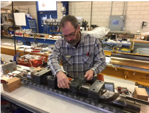
Coil lead splicing, epoxy impregnation
