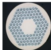
0.7 mm RRP108/127 40-strand cable with SS core
