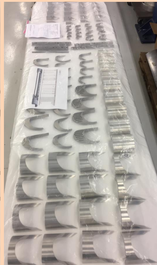
Ti poles and spacers, SS saddles
