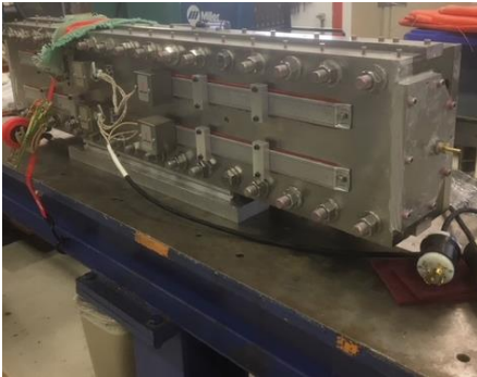
Coil lead splicing, epoxy impregnation
