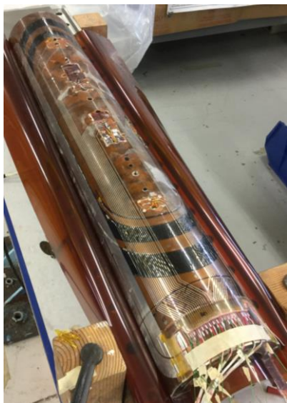
Traces on outer coil OD
