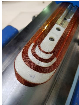
First layer winding and polymerisation
