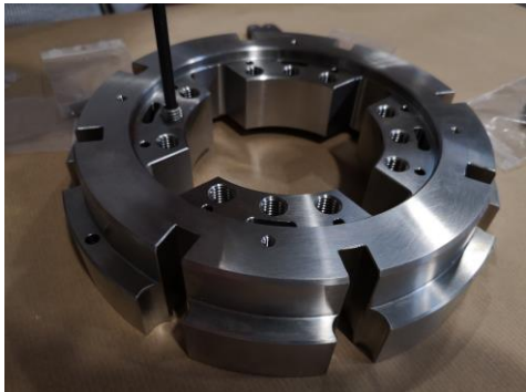
Longitudinal prelaod apply with instrumented bullets
