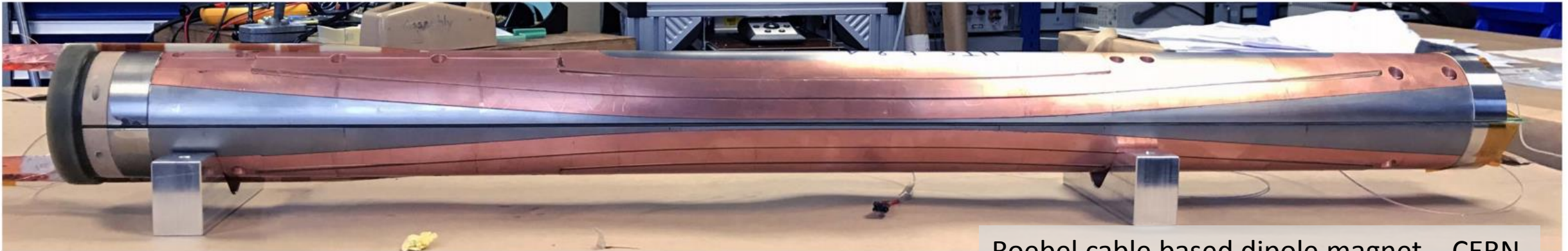
Roebel cable based dipole magnet – CERN
