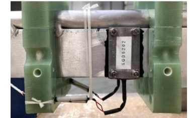
Superconducting Quench Detector (developed at CERN)
