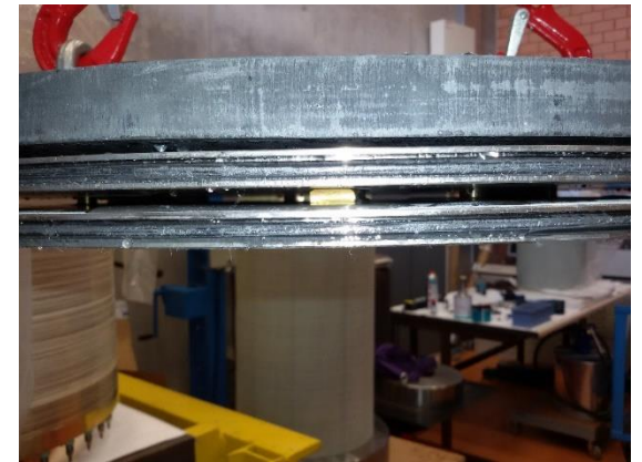
Mock-up test hydraulic bellow
