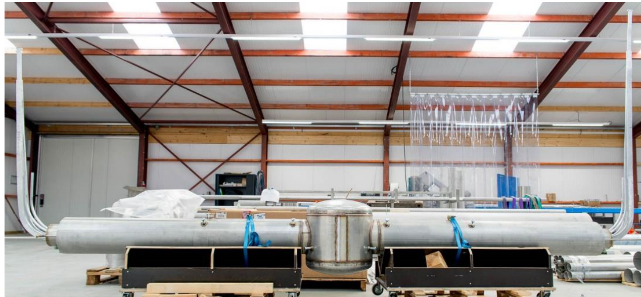
Superconducting Quench Detector (developed at CERN)
