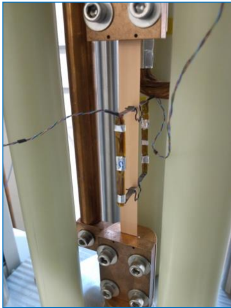
Axial tensile RT or 77K w/ I_c
