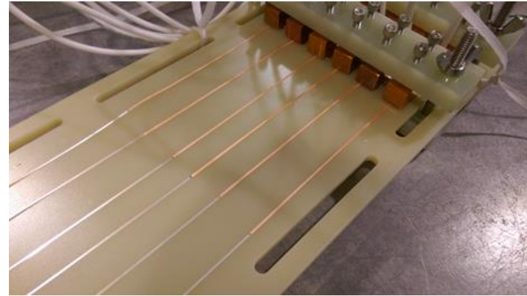
Selective Cu plated 1mm tapes under I_c test
