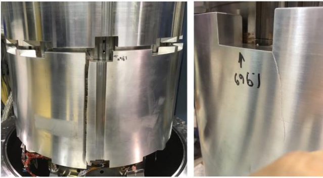
Fig. 6. MQXFAP2 nonlead end shell cracks, which all originated at corners of the alignment cut-outs. Photo is courtesy of D. Cheng, LBNL.
