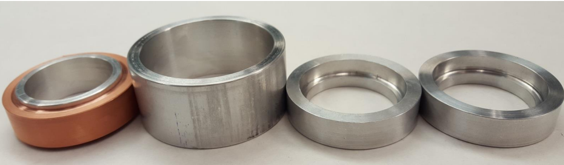
28AUG17 – Al Extended Outer Ring (25.4 mm) and 2 Pistons
