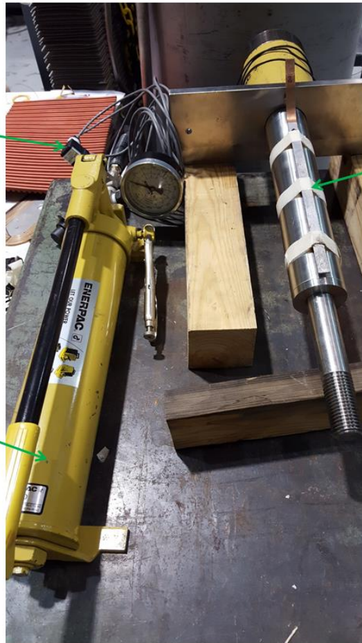
COMPRESSION FIXTURE SETUP
