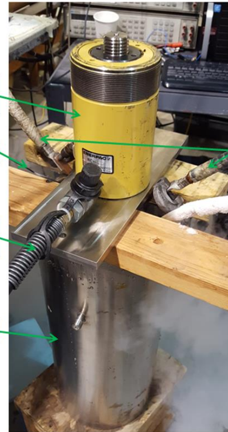
COMPRESSION FIXTURE SETUP IN OPERATION
