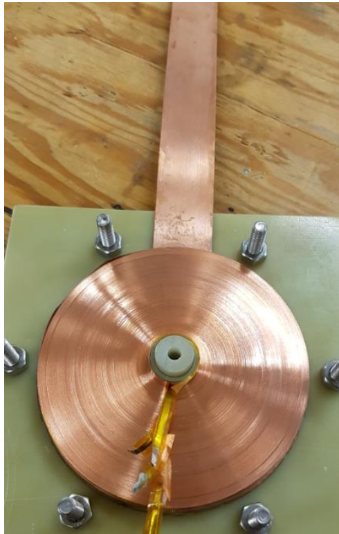
Both-side-Insulated copper cooling disk
