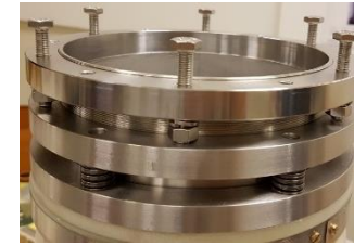
For a coil's elastic behavior during cooling and operation
