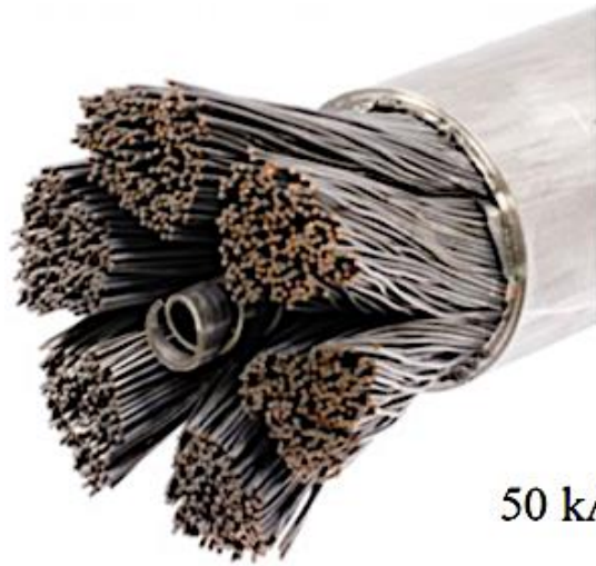
wire bundle within an ITER TX cable
