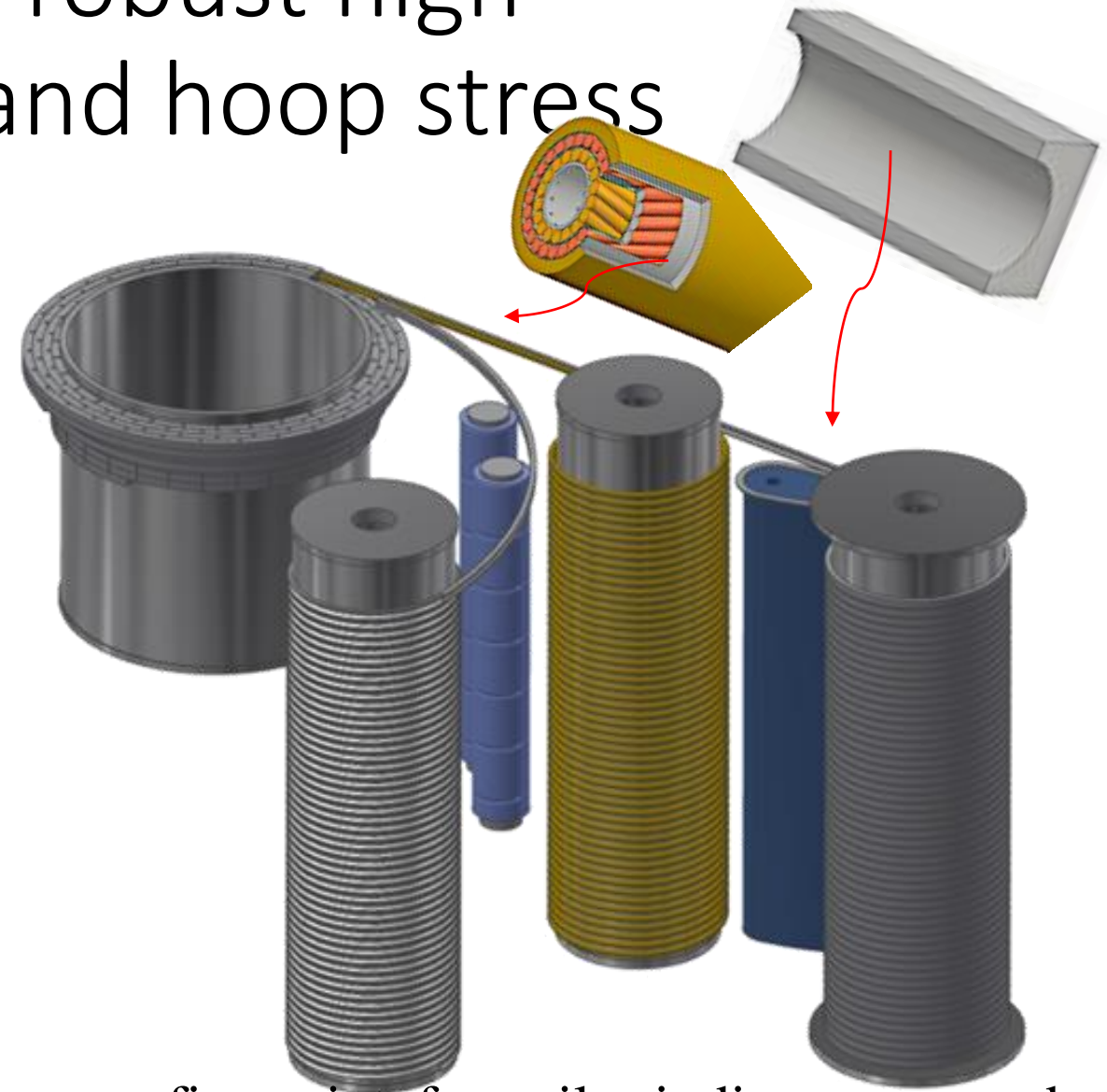
configuration for coil-winding co-wound armored SuperCIC for a solenoid winding.
