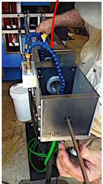
draw sheath tube onto cable.
