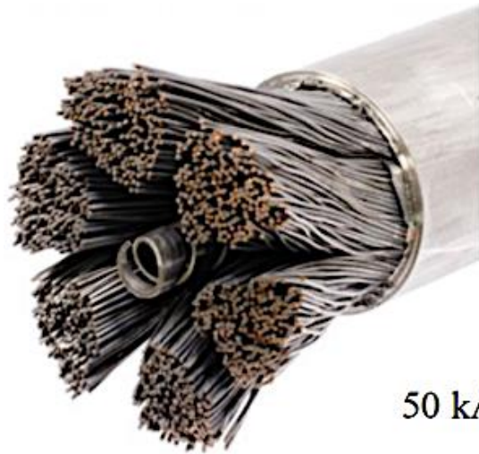
wire bundle within an ITER TX cable
