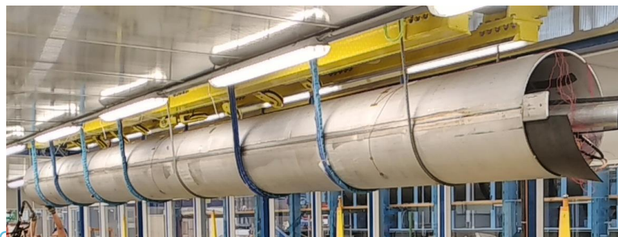
F. Lackner, et al. “Assembly of MQXFBP1 prototype, the Nb 3 Sn Q2 quadrupole for HL-LHC”, this session
