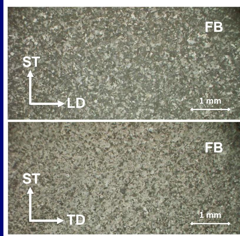
↑ Example of results of macrographic examination of a sample issued from the forging for the FB. Longitudinal Direction (LD) that coincides with the direction of maximum flow, Transverse Direction (TD) and Short Transverse (ST) direction are identified. The macrostructure is homogeneous within the cross sections, due to the lack of segregation and homogeneous grain size.
