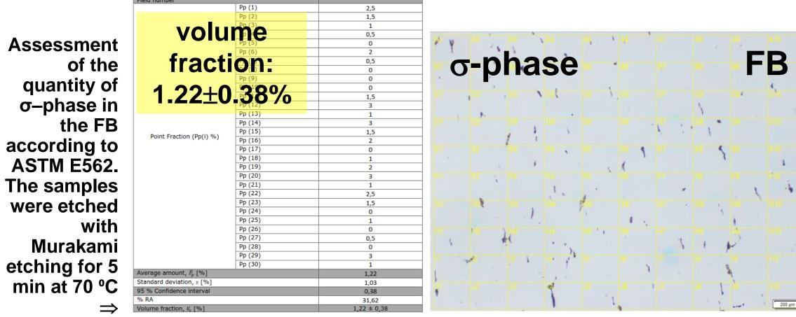
$\Leftarrow$  Distinctive appearance of  $\delta$ -ferrite and  $\sigma$ -phase following a Murakami etching (#98 as per ASTM E407). The latter colors not only the  $\sigma$ -phase in blue, but also  $\delta$ -ferrite in yellow/brown. Therefore, taking into account that for austenitic stainless steel, the preferential location of precipitation of  $\sigma$ -phase is the austenite – ferrite interface, it is very common to find the secondary phases mixed together.
