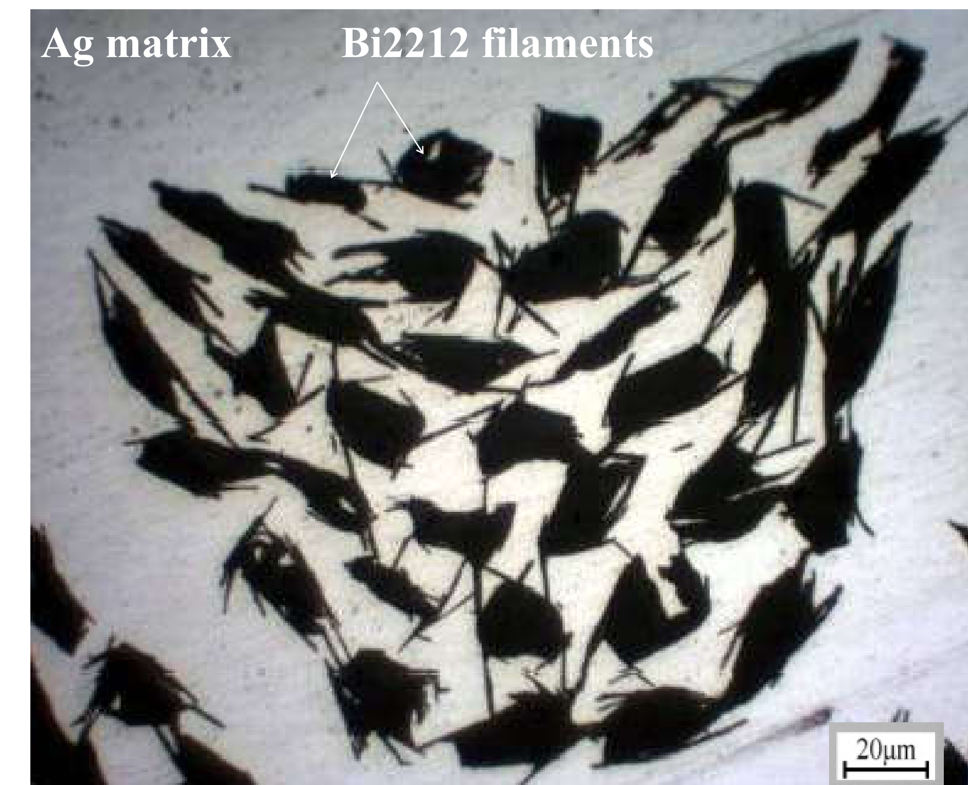
SEM image of the filaments after melt-processing with 5Mpa pressure
