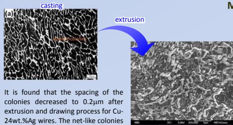
It is found that the spacing of the colonies decreased to 0.2μm after extrusion and drawing process for Cu-24wt.%Ag wires. The net-like colonies have been broken up into smaller net structure during the process.
