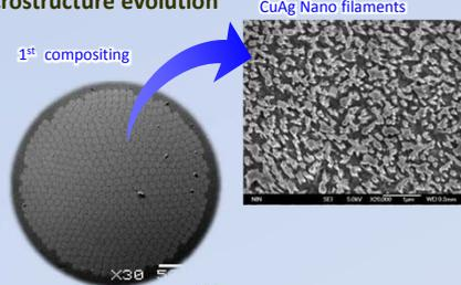
The net-like junctions have transformed to single nano-fibers. In compared with eutectic in Cu-Ag casting alloys, eutectic filaments in microcomposites distribute more regularly and the size is below 40nm.
