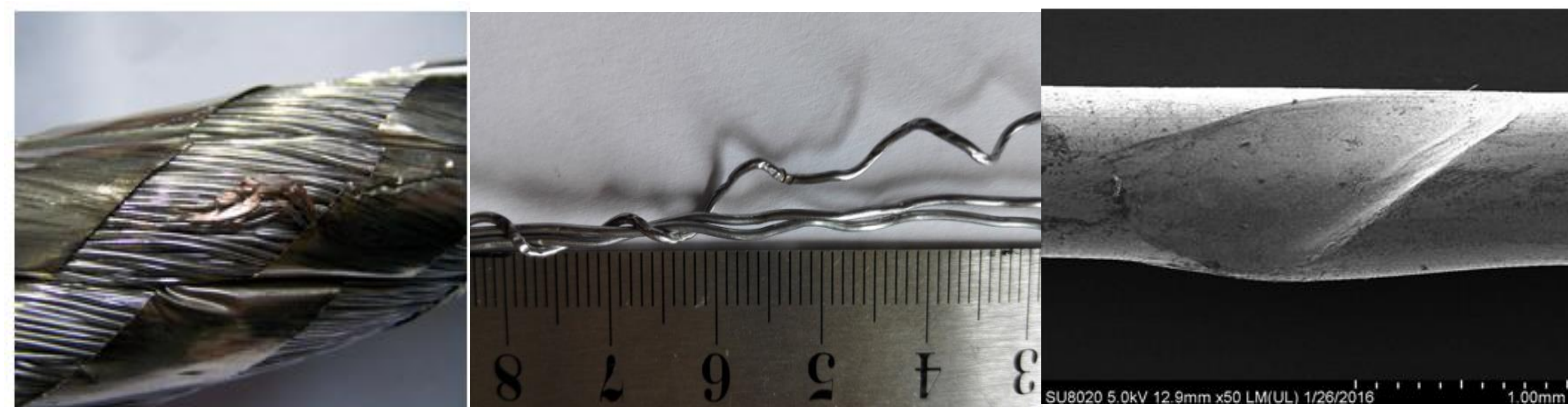
Fig. 2. Damaged of Nb3Sn strand
