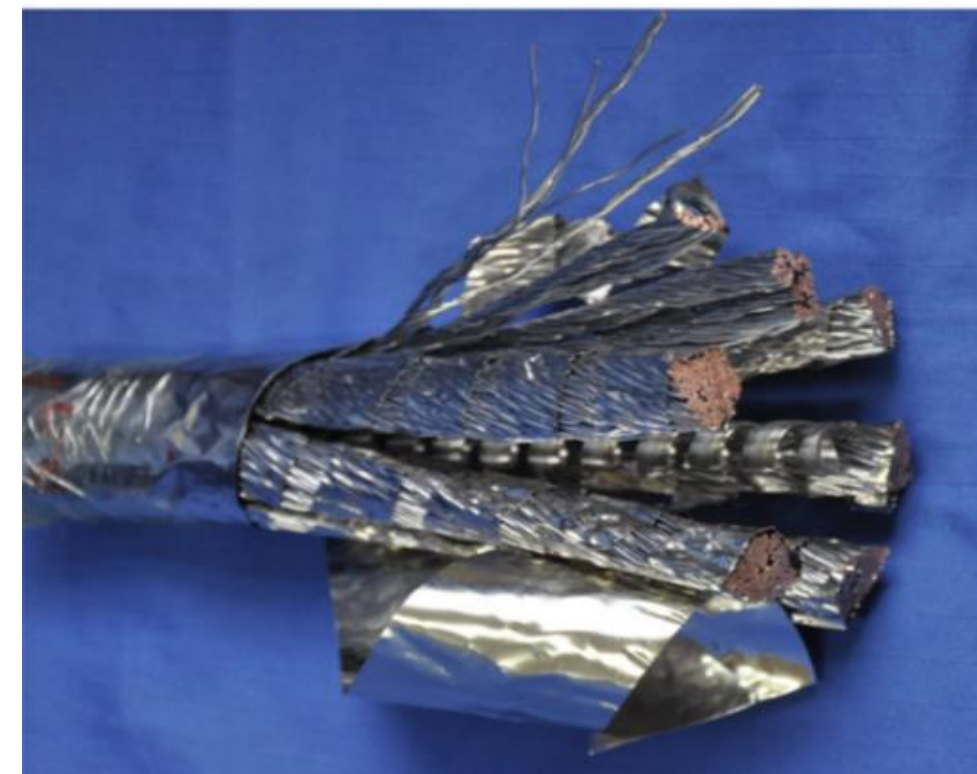
Fig. 1. lay out of disassembled cable
