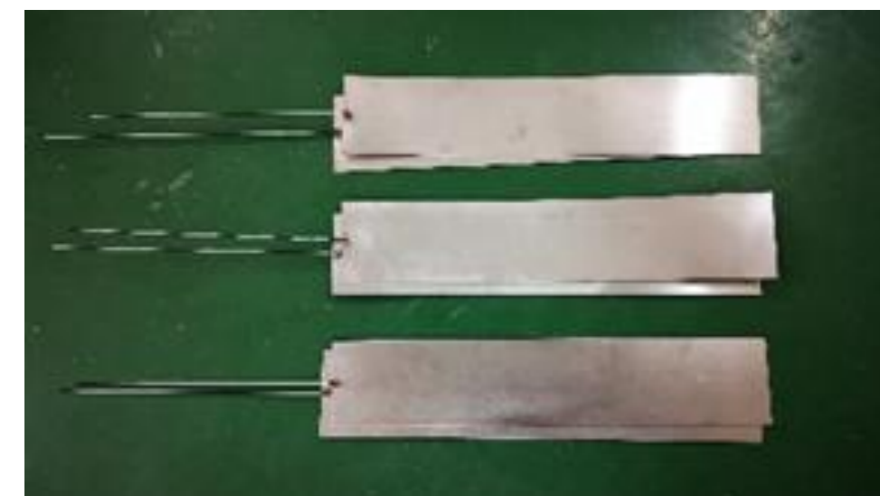
Fig 2. Home-made bladders with stainless-steel sheets by continuous laser welding
