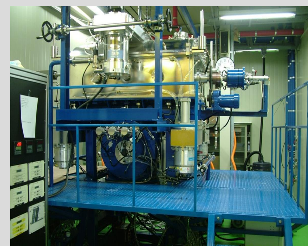
Fig. 1. The photograph of EDDC installed in KERI (Drum style : sample holder for 100m tape , 50cm diameter: 50cm, length: 72cm )
