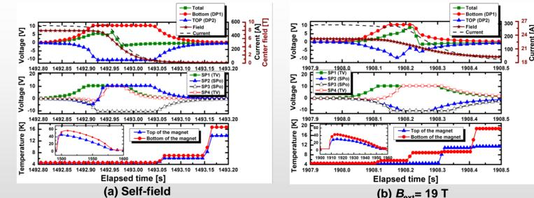
Fig. 9. Quench behaviors of the MI insert
