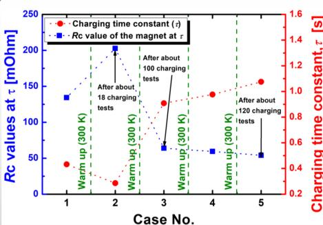
Fig. 7.  $R_c$  values of the MI insert with respect to several warm-up events.
