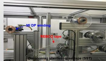
Fig. 2. MI double-pancake (DP) coil wound by LNCMI homemade HTS winding machine
