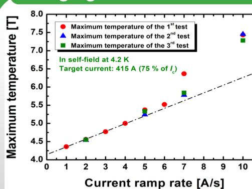
Fig. 10. Maximum temperature values of the TV-SPo insert with various ramp rates at 4.2 K in self-field.
