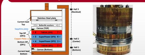
Fig. 5. Instrumentation diagram and picture of the insert
