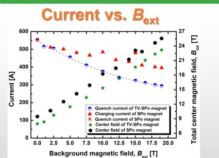
Fig. 8. Quench, charging currents and total center magnetic fields of a TV-SPo and only SPo insert under various  $B_{ext}$  at 4.2 K.
