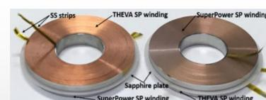
Fig. 3. A photograph of the MI REBCO DP coils
