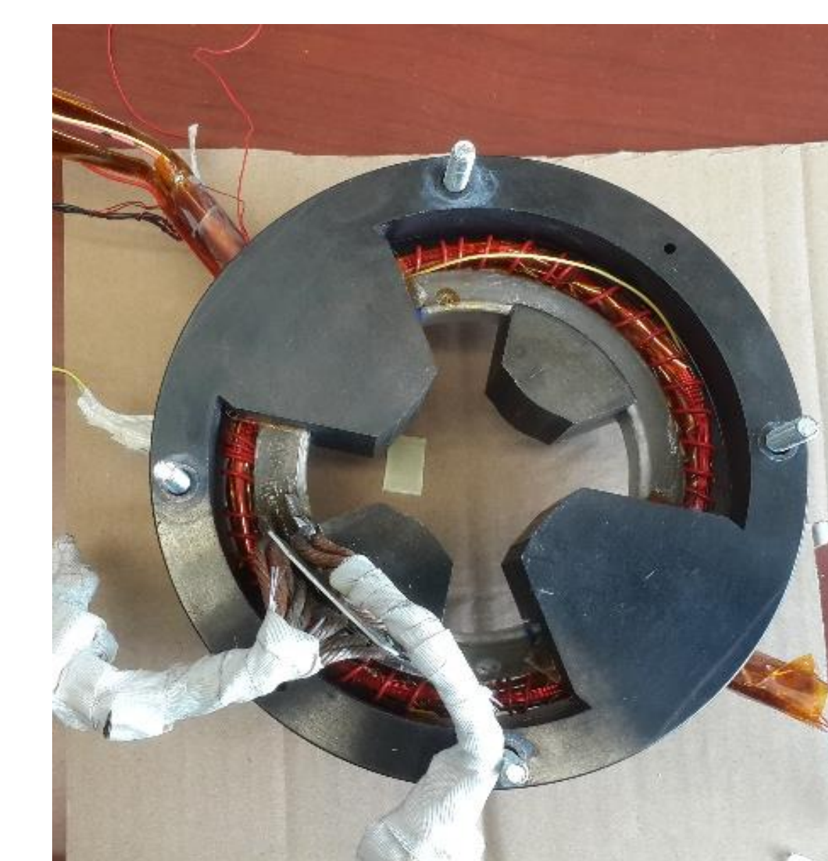
Quadrupole magnet with HTS primary and secondary coils
