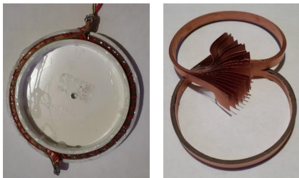
Fig. 2. Tested HTS coils with outer ends (left) and inner ends (right).
