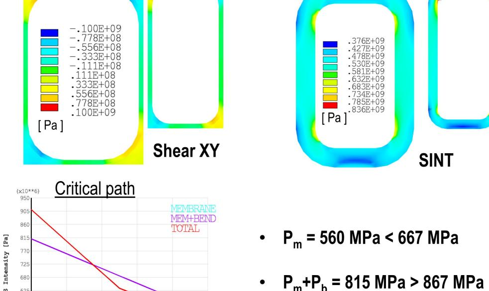
Shear stress on turn insulation: the obtained values are critical. Further studies have been done in order to verify the integrity of the structure and ensure electrical insulation between the cables. In depth analyses have been computed drawing on Puck's criterion. The critical zone remains in the A-zone of the Puck curve, in which the crack is expected to remain interlaminar.
