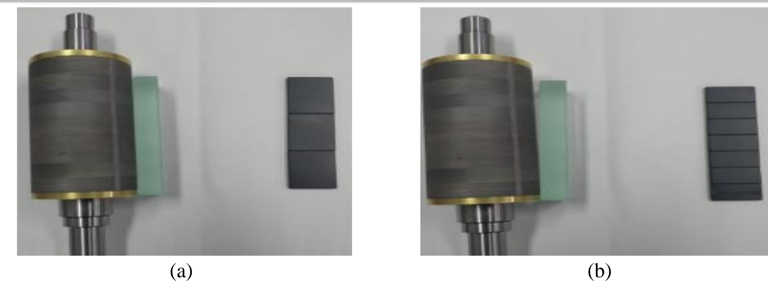
Fig. 6. Segmented magnet actual image (a) three-segment magnets (b) seven-segment magnets
