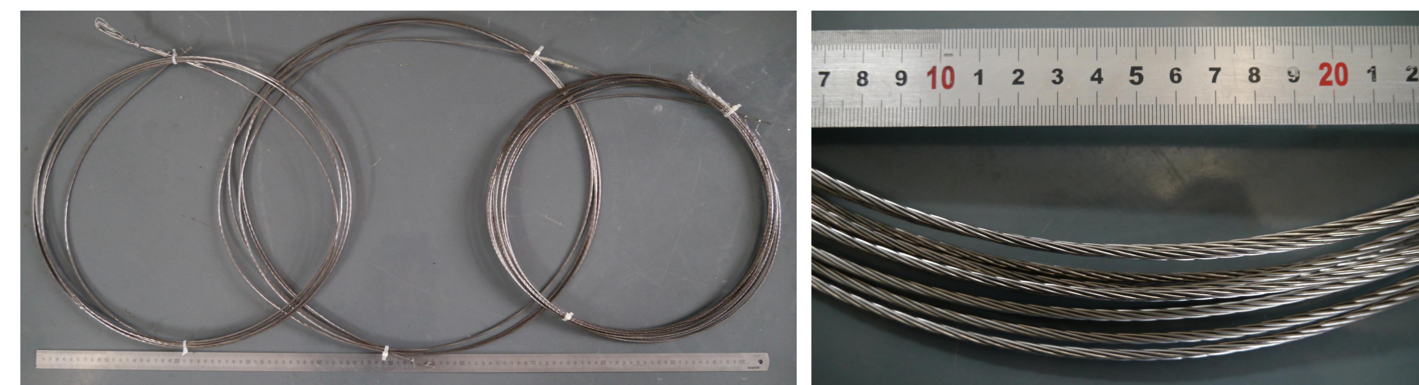
Fig. 3. (a) Three fabricated superconducting cables (b) Cable details
