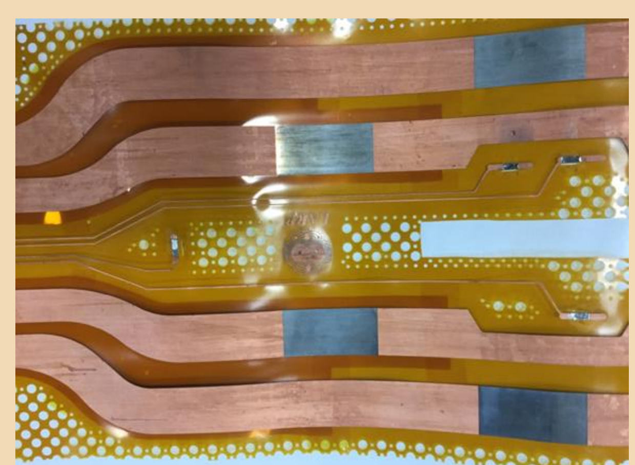
Fig. 2 MQXFA quench heater trace
