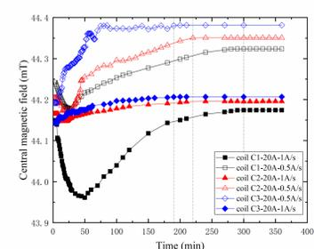
Fig. 5. The central magnetic field waveforms of the Coil C1, Coil C2 and Coil C3 charge test. Coil C1 (■, □), Coil C2 (▲, △) and Coil C3 (◆, ◇).
