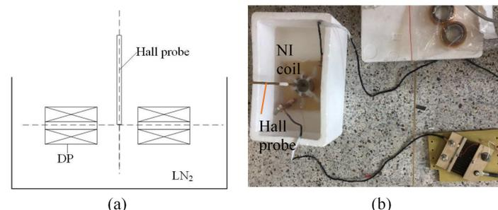
Fig. 3. The schematic diagram and view of coil test. (a) Schematic view, (b) Photo of test arrangement.
