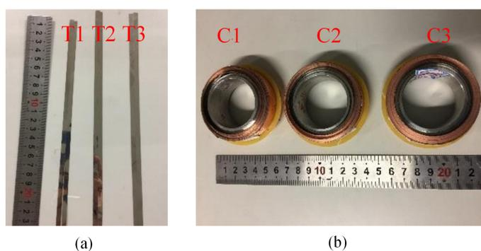
Fig. 1. Photograph of three NI HTS coils. (a) Non-treated SS tape T1, chemical treated SS tape T2, and thermal and chemical treated SS tape T3. (b) The NI HTS DP coils C1, C2 and C3.
