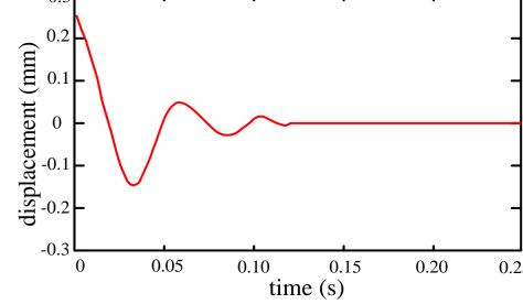
The magnetic flux density between the rotor and the magnetic poles satisfy the design requirements The initial position of rotor is assumed as (0.25) mm, 0). Once the rotor is active, the rotor returns to the equilibrium position within 0.13 s.
