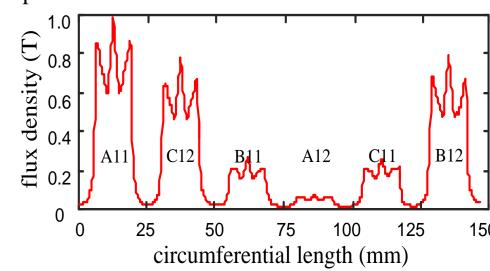
The maximum magnetic flux density between the each magnetic pole named A11 and rotor is about 0.8 T and the minimum magnetic flux density between the magnetic pole named A12 and rotor is about 0 T.
