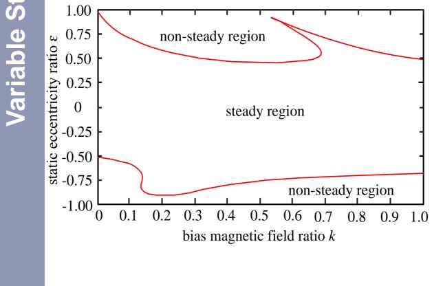
It can be seen that the variable stiffness coefficient K of the sixpole AC HMB is related to the static eccentricity ratio  $\varepsilon$  and the bias magnetic field ratio k.
