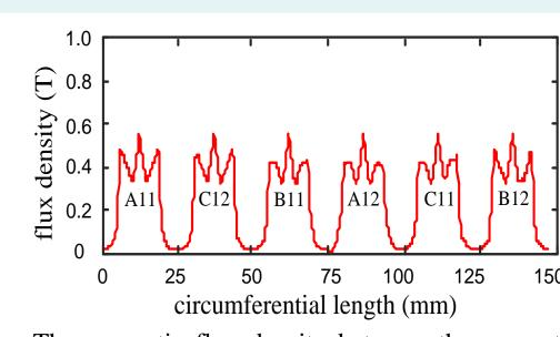
The magnetic flux density between the magnetic pole and rotor is about 0.4 T.
