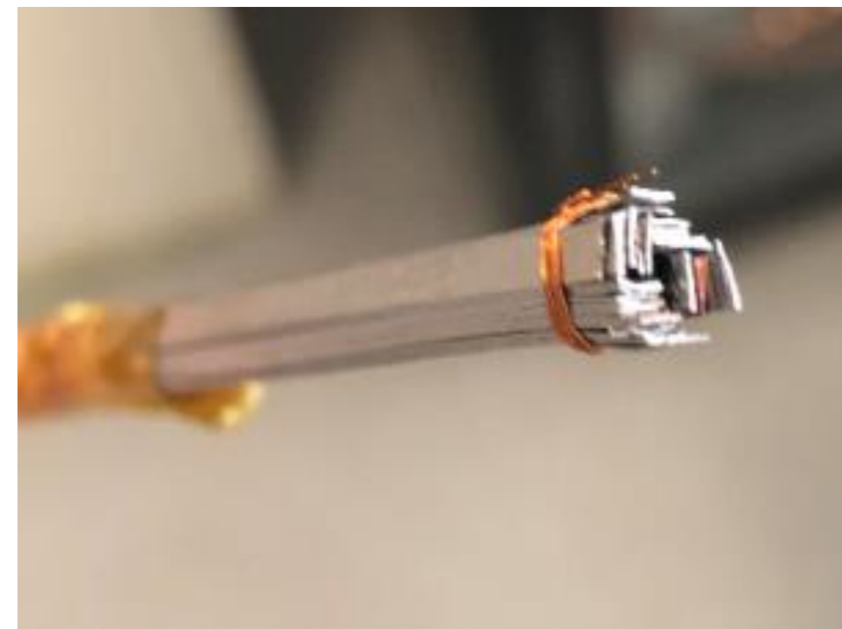
Fig. 1 (a) Cross-section view of the quasi-isotropic superconducting strand. The total cross section of the strand is 5 mm × 5 mm, and the cross section of the tapes is 4 mm × 4 mm. The thickness of copper sheath is 0.4 mm, and the thickness of the aluminum foil is 0.1 mm. (b) The terminal view of the quasi-isotropic strand. The number of YBCO tapes is 72
