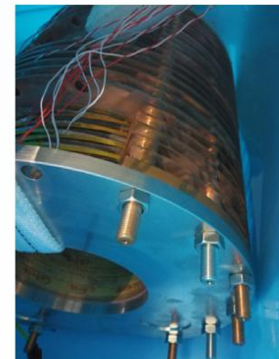
Fig.8 Magnet in the LN_2 tank
