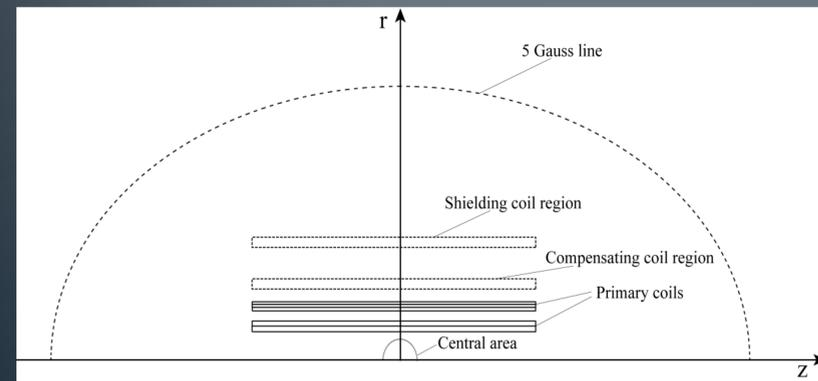
Fig.1 Diagram of the compensating field method for high-field superconducting magnet design
