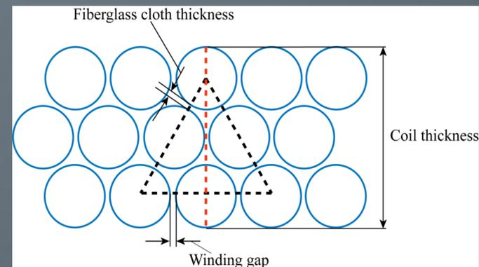
Fig. 2 A sketch map of the round superconducting layout in a NMR magnet coil.
