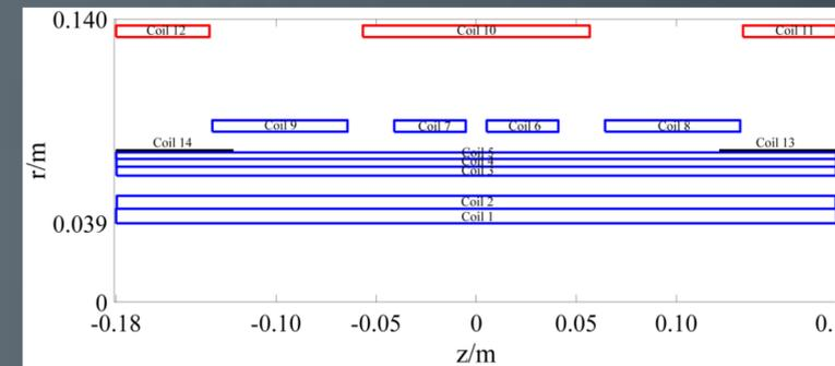
Fig. 3 Coil pattern of a 7T conduction-cooled NMR superconducting magnet
